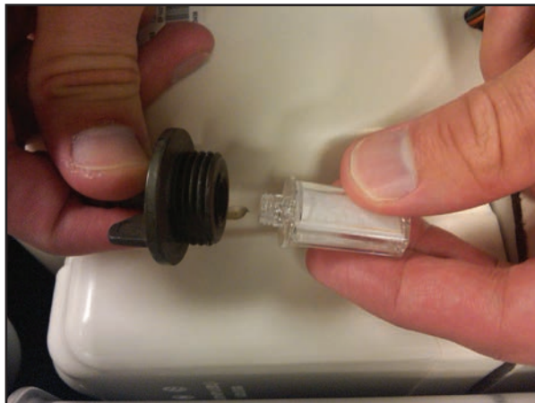
Figure 22: Installing the new HEPA Filter.
