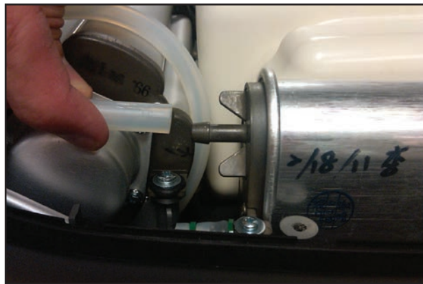
Figure 19: Tubing on Filter Carriage.
